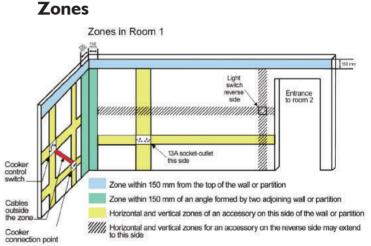
Electrical regulations refer to cable zones which indicate potential cable positions placed in a wall, this allows an end user to be aware of safe locations where a picture or a hole can be drilled. See diagram above.
