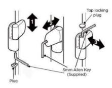
2. Horizontal adjustment: for setting the correct distance between leaves and the weather seal cover (8mm).
