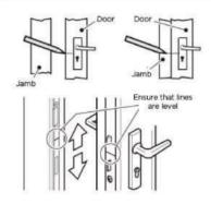
The lock and keep have an alignment line scored on them, these need to be aligned to ensure correct operation.
